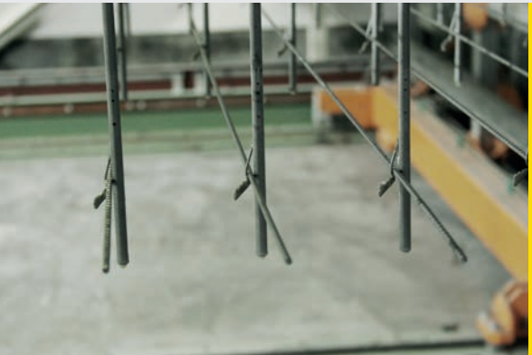
Clip system for automatic insertion of the loose bars
