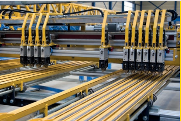
Gridless production of bespoke mesh and reinforcement cages
